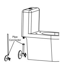
a. Without flexible pipe:unscrew the pipe connectorb. With flexible pipe:take off the water supply pipeand then place the flexible pipeinstead
