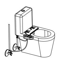
Connect hot water tube to hot water inlet of the bidet, and connect cold water tube to cold water inlet of the bidet
