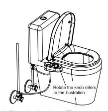
Adjust the knob as illustrated, turn on the angle valve and then check if there is any seepage and leakage for each joint
