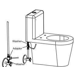
Connect the adaptor to the water supply pipe
