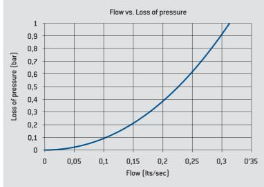
Hydraulic characteristics obtained according to EN 1267.
